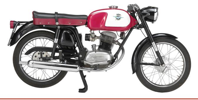
The displacement of this model, derived from checca 98 GTES, had been increased to 123cc. Production started in October 1962. It was essentially the same bike as the Checca 98, but wiyh the increase in power, the race results on mixed tracks were stellar. Because the bike was succesfully mixed high quality with a lower price (185.000 Lire) sales were impressive; 1.500 units were built.
