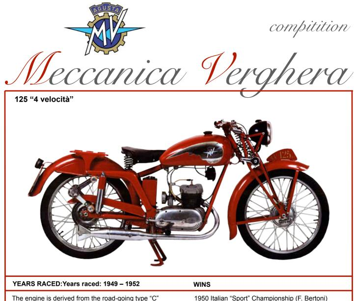
The engine is derived from the road-going type "C" and has a high performance cylinder. It debuted victoriously on the 27th of March 1949 on the circuit of Lodi (F.Bertoni). The engine was also used on "Race Scooters" in track, endurance and hill climbing events.
